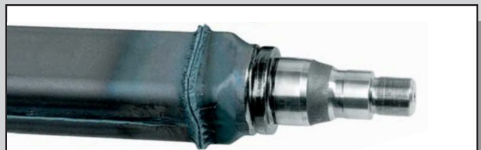
Axle beam after flash butt-welding
